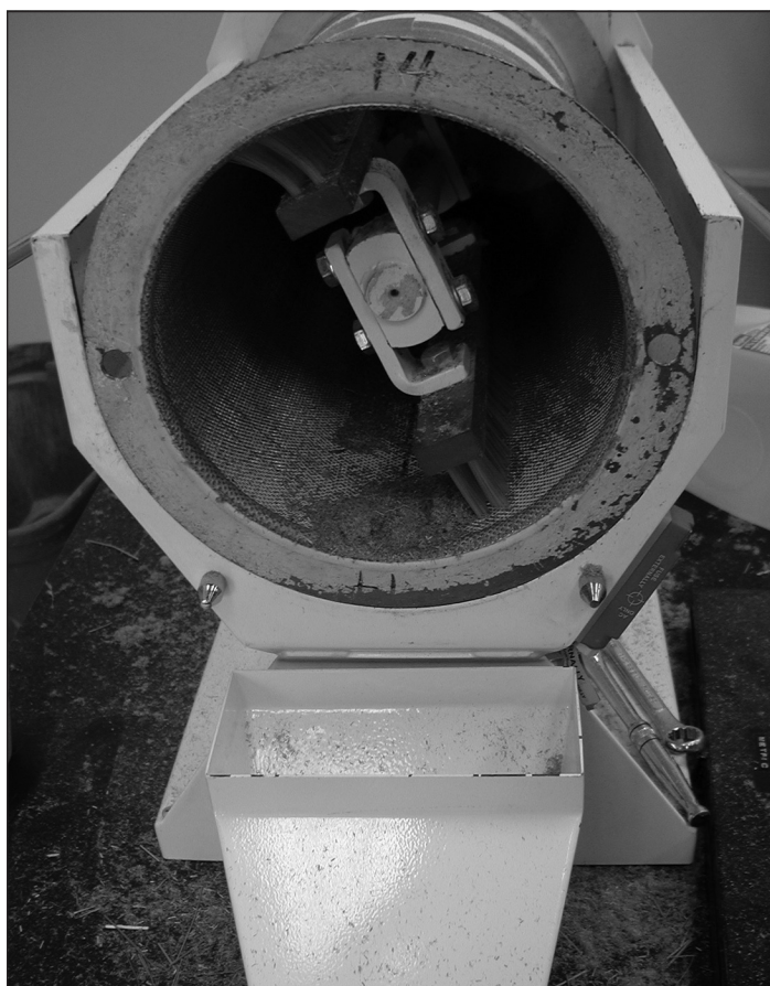
Westrup Lab Scarifier/Brush machine with housing removed to show brushes and drum screen.
